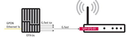
Application with EFX-14 DPU/ONU: existing Router kept in place — future proof solution
