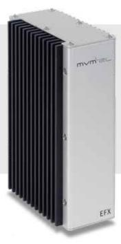
The **EFX-11** is a single Fiber-extender, based on G.fast technology, allowing to address FTTB/FTTdp deployment for each customer individually. There is no media, equipment or even power sharing. Each subscriber reverse-powers his own equipment over the same copper pair that is used for high speed data. Such clean situation enables easiest and fastest deployment of Premium Triple Play Services.
